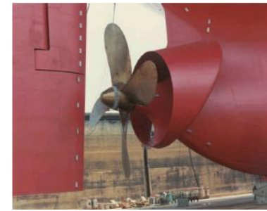
Wake equalizing duct
