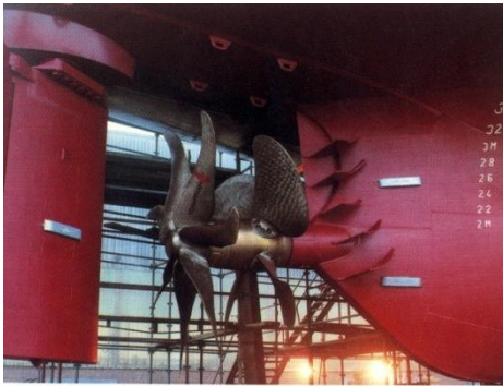
Combination of vane wheel & hydrodynamic fin system
