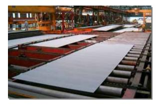
Condition in a subcontractor 's shop Steel : Occasionally C or D plates Salt : 30~270mg/m2 (Before blasting) 20~80mg/m2 (After blasting) Other contaminations; Oil, mill scale and rust are found. Blasting grade : Partly less than Sa 2.5
